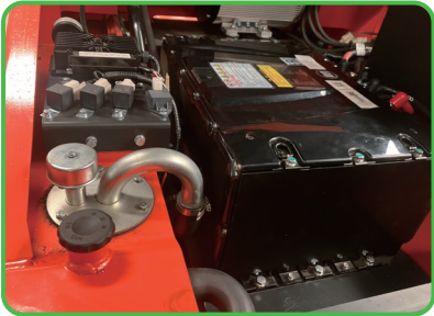
Convenient hydraulic oil level check.
